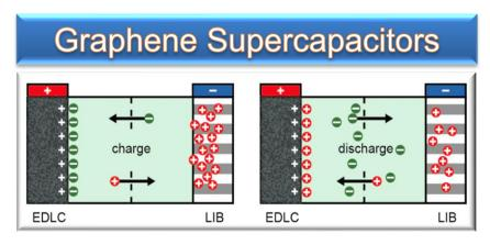
➢ Higher Energy density was always a pain point for supercapacitors (EDLCs). Secure Supplies uses a mixed Lion-ion electrolyte technology to increase the energy density of Graphene Supercapacitors up to 150Wh/Kg, which provides Better Energy Storage Solutions to Replace traditional batteries.
